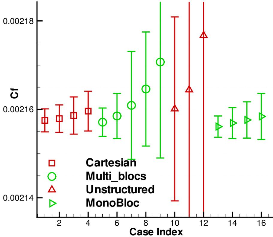
Figure 2: Friction resistance coefficient for the top wall.
