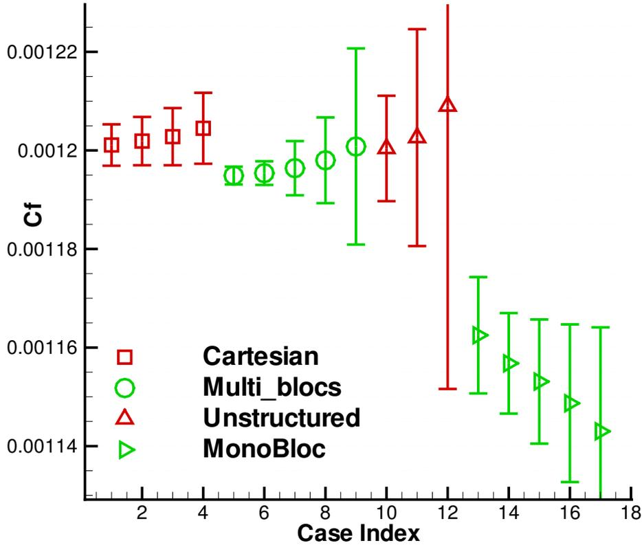
Figure 3: Friction resistance coefficient for the bottom wall.
