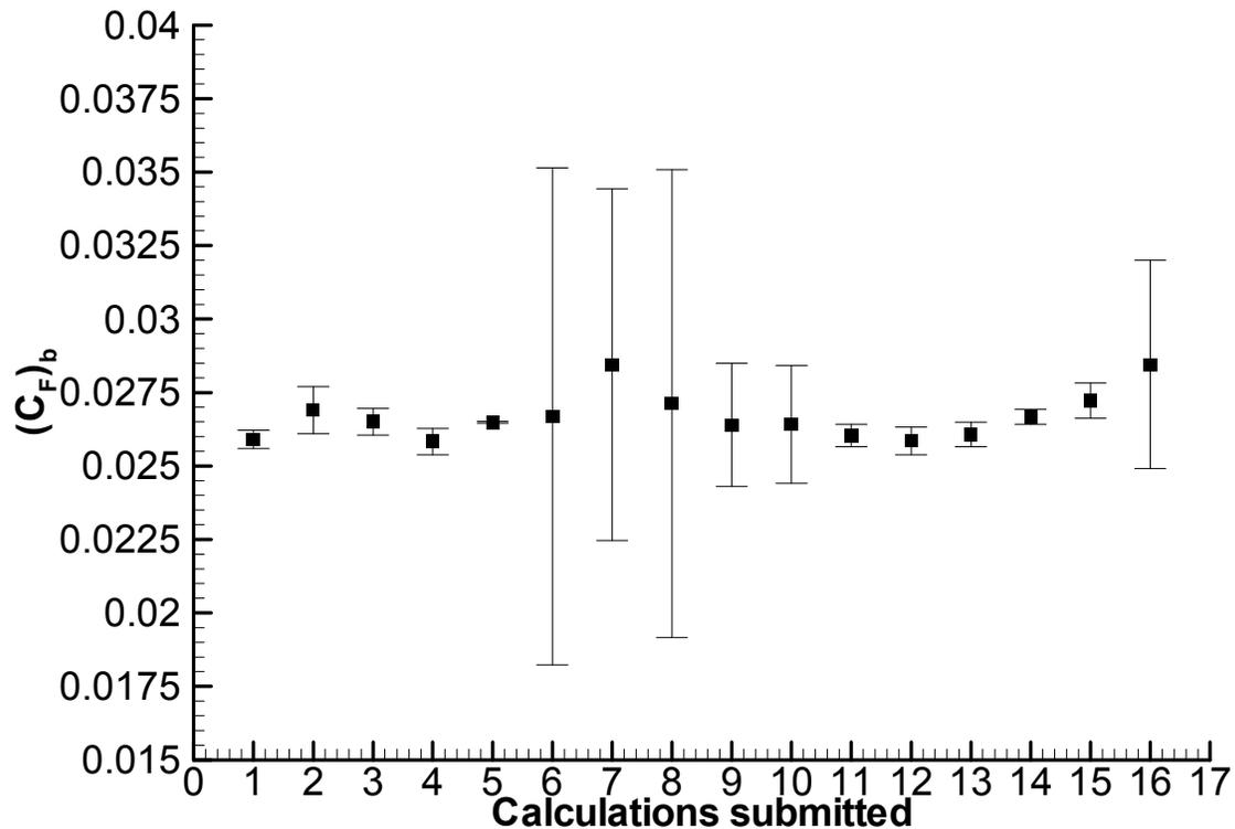
Figure 2: Friction force on the bottom boundary in the backward-facing step flow (ERCOFTAC C-30)
