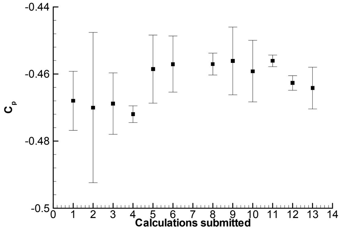
Figure 1: Pressure at  $x=2.5h$  and  $y=0.25h$  in the flow over a hill (ERCOFTAC C-18)
